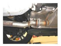
3) Using a 13mm socket, unbolt the left tailpipe assembly at the flanged connection at the rear of the muffler. Slide the three hanger rods out of the rubber mounts on the vehicle and remove the left tailpipe assembly.
