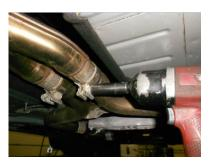
4) Support the rear of the system with a stand, then starting at the rear of the vehicle remove the three hangers on the right side of the system from the rubber mounts on the vehicle. Unclip the ground strap from the middle hanger on the right tailpipe and using a 15mm socket loosen the clamps at the slip fit connections behind the catalytic converters. Then with the help of an assistant, lower the stand and slide the system back off of the head pipes. Carefully lower from the vehicle.
