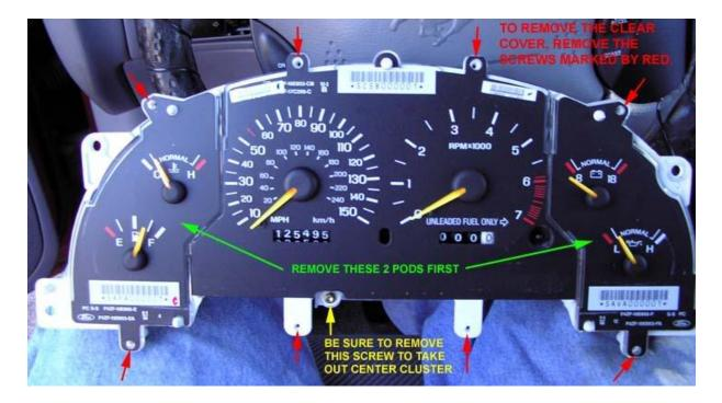
You will need to gently pry under the face of each gauge cluster to remove, using a flat blade screwdriver. It is best to remove the left and right gauge clusters first and then the speedometer. The gauges are held into place by electrical studs that press through electrical contact sleeves.
