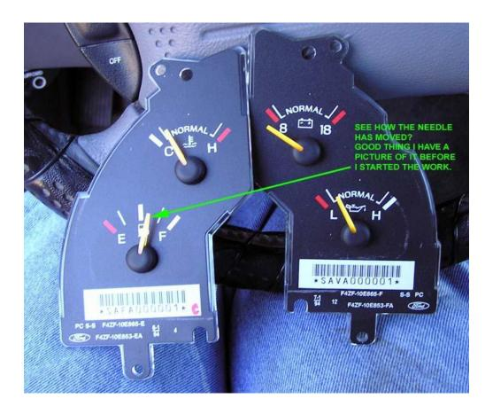
The gauges will synchronize once reinstalled and the ignition switch is switched on.
