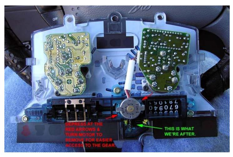
When trying to remove the motor you may either have to depress or lift up on the plastic tabs.
